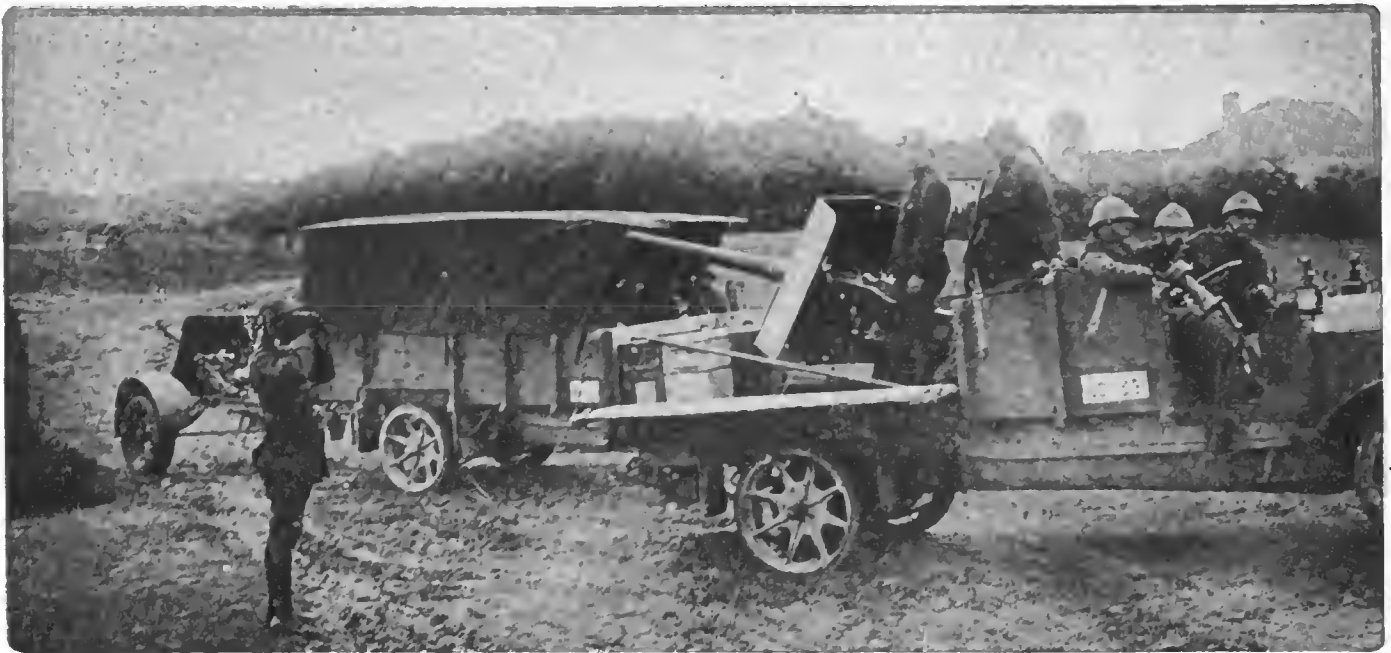
Belgian light field pieces used in connection with motor trucks. Note the steel wheels required by their weight
